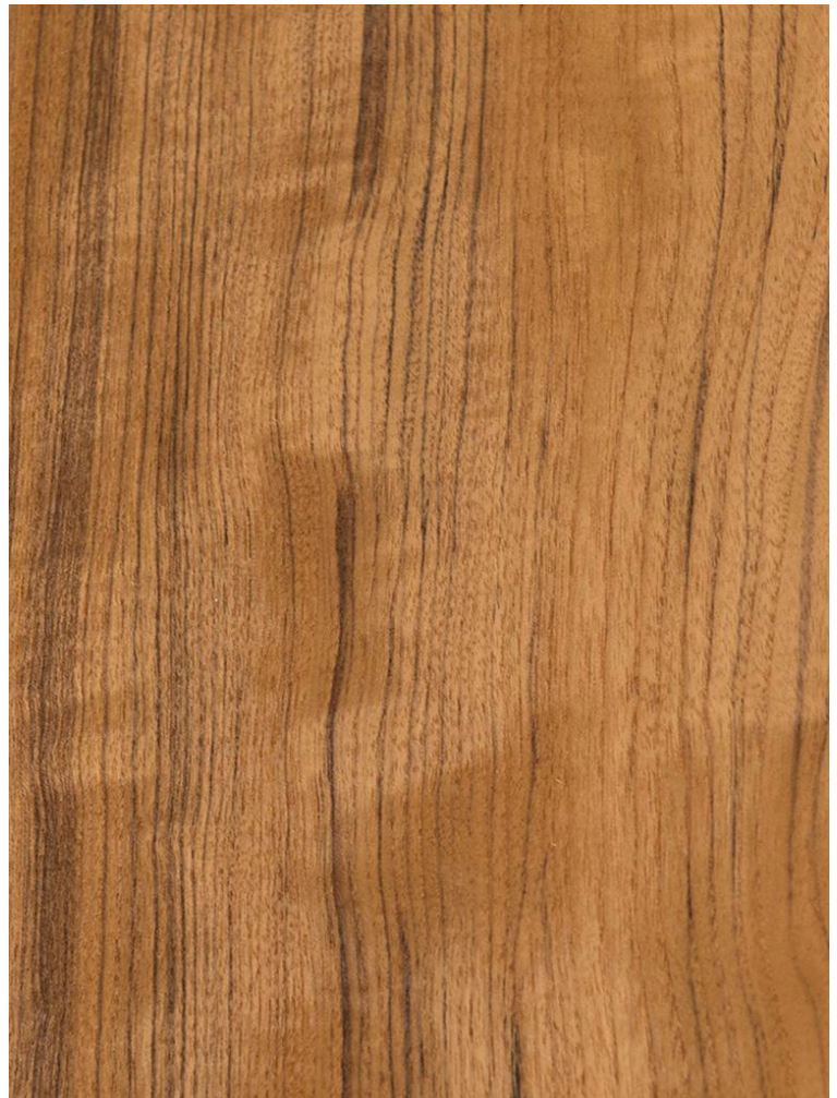
ABOVE: QUARTERED FIGURED TEAK. BELOW LEFT: TEAK IN A SLIP MATCH. BELOW RIGHT: TEAK IN A BOOK MATCH.
