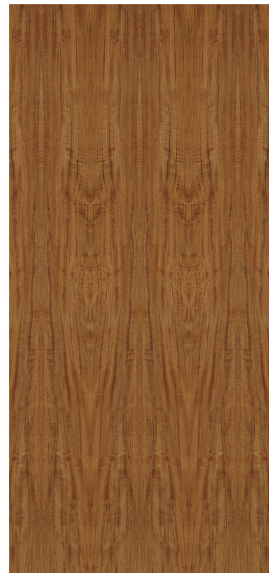
ABOVE: QUARTERED FIGURED TEAK. BELOW LEFT: TEAK IN A SLIP MATCH. BELOW RIGHT: TEAK IN A BOOK MATCH.
