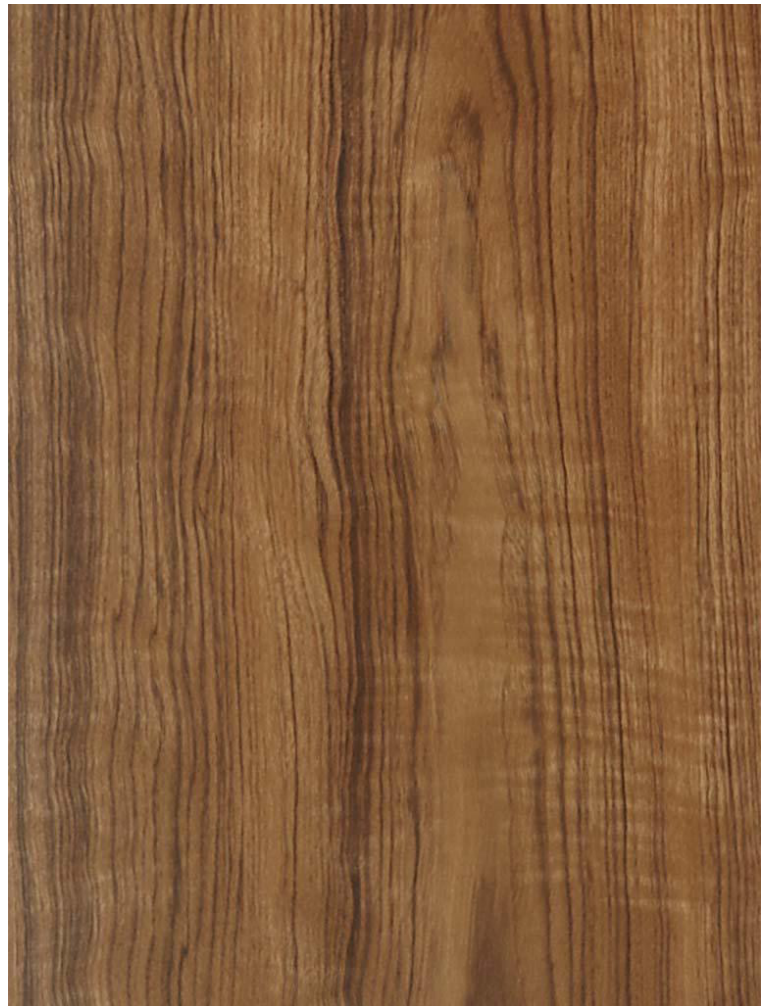
ABOVE: FLAT CUT FIGURED TEAK. BELOW LEFT: TEAK IN A SLIP MATCH. BELOW RIGHT: TEAK IN A BOOK MATCH.
