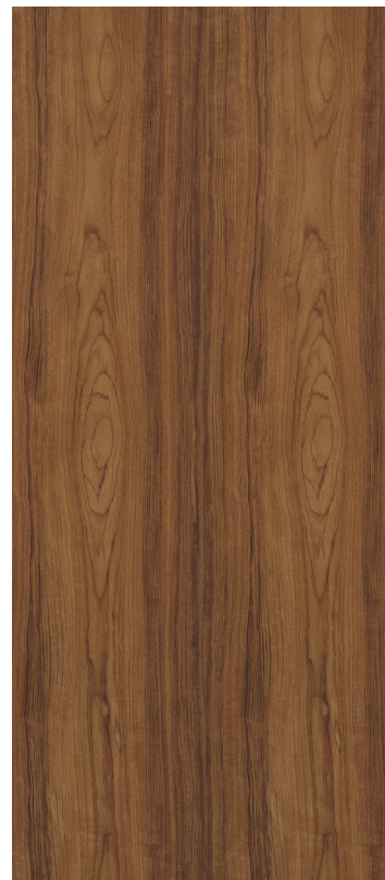
ABOVE: FLAT CUT FIGURED TEAK. BELOW LEFT: TEAK IN A SLIP MATCH. BELOW RIGHT: TEAK IN A BOOK MATCH.
