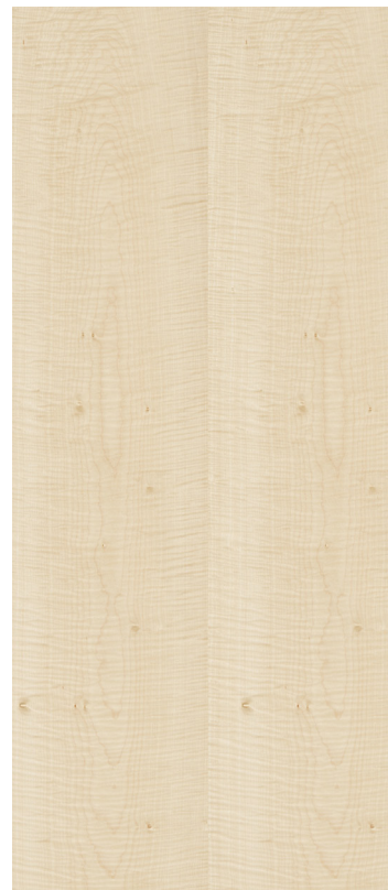
ABOVE: FLAT CUT FIGURED SYCAMORE. BELOW LEFT: SYCAMORE IN A SLIP MATCH. BELOW RIGHT: SYCAMORE IN A BOOK MATCH.
