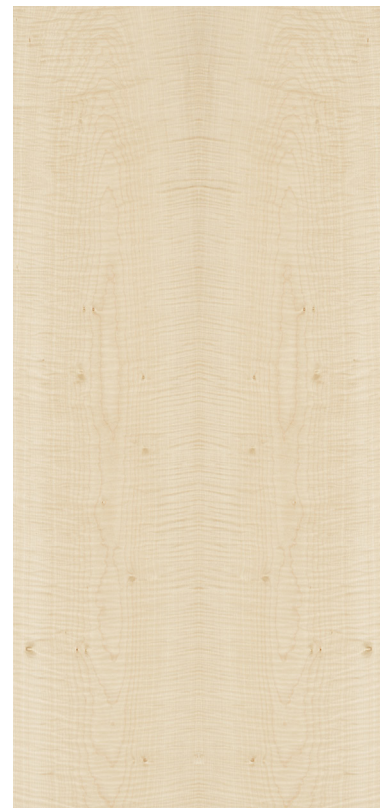
ABOVE: FLAT CUT FIGURED SYCAMORE. BELOW LEFT: SYCAMORE IN A SLIP MATCH. BELOW RIGHT: SYCAMORE IN A BOOK MATCH.
