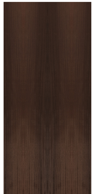
ABOVE: QUARTERED FUMED SAPELE. BELOW LEFT: SAPELE IN A SLIP MATCH. BELOW RIGHT: SAPELE IN A BOOK MATCH.
