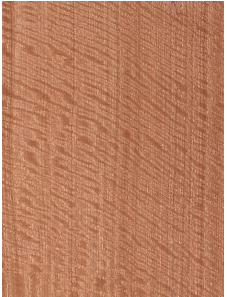
ABOVE: QUARTERED FIGURED SAPELE. BELOW LEFT: SAPELE IN A SLIP MATCH. BELOW RIGHT: SAPELE IN A BOOK MATCH.
