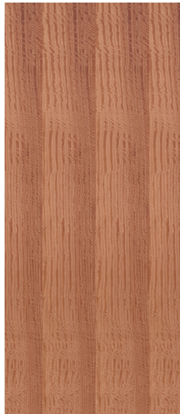
ABOVE: QUARTERED FIGURED SAPELE. BELOW LEFT: SAPELE IN A SLIP MATCH. BELOW RIGHT: SAPELE IN A BOOK MATCH.
