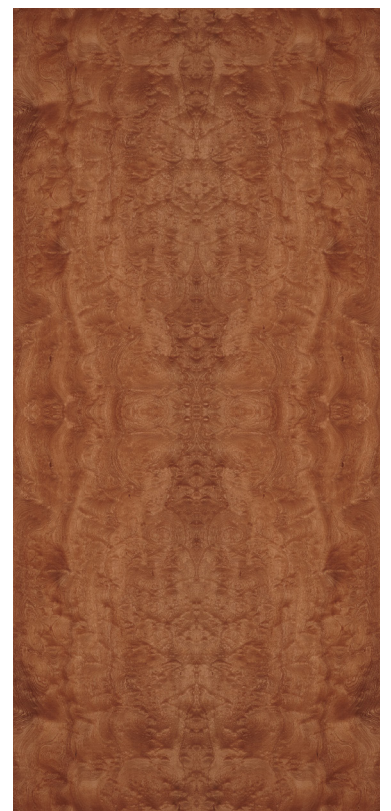
ABOVE: POMMELE SAPELE. BELOW LEFT: SAPELE IN A SLIP MATCH. BELOW RIGHT: SAPELE IN A BOOK MATCH.
