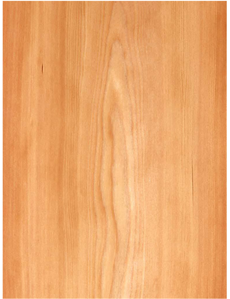
ABOVE: FLAT CUT LARCH. BELOW LEFT: LARCH IN A SLIP MATCH. BELOW RIGHT: LARCH IN A BOOK MATCH.
