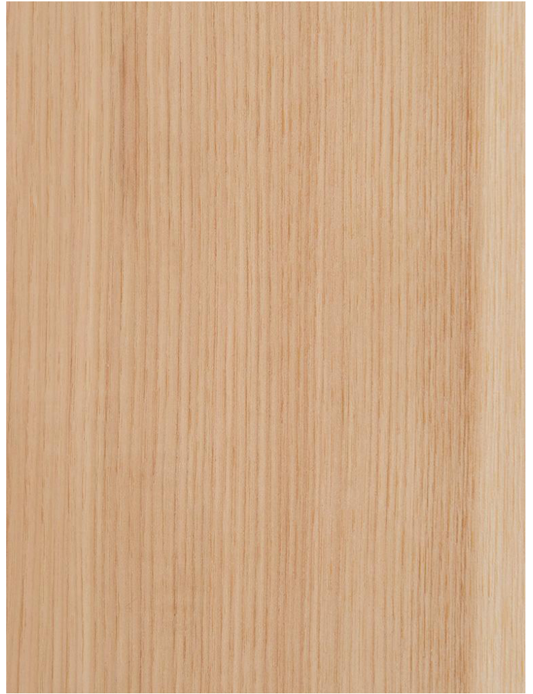
ABOVE: QUARTERED PLAIN HICKORY. BELOW LEFT: HICKORY IN A SLIP MATCH. BELOW RIGHT: HICKORY IN A BOOK MATCH.
