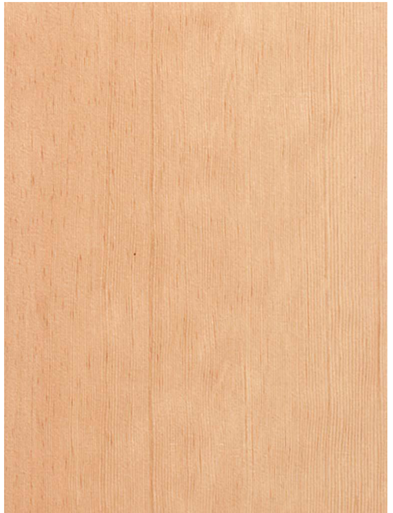
ABOVE: QUARTERED DOUGLAS FIR. BELOW LEFT: DOUGLAS FIR IN A SLIP MATCH. BELOW RIGHT: DOUGLAS FIR IN A BOOK MATCH.
