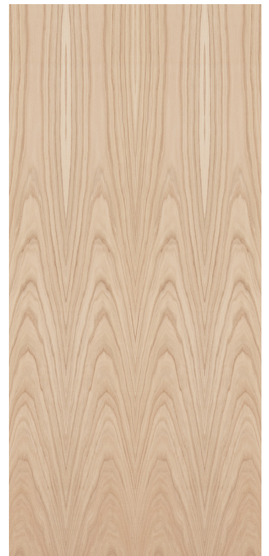
ABOVE: FLAT CUT EUROPEAN CHESTNUT. BELOW LEFT: CHESTNUT IN A SLIP MATCH. BELOW RIGHT: CHESTNUT IN A BOOK MATCH.
