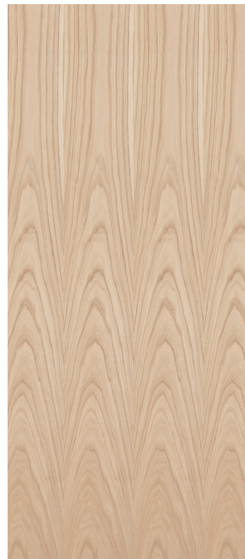
ABOVE: FLAT CUT EUROPEAN CHESTNUT. BELOW LEFT: CHESTNUT IN A SLIP MATCH. BELOW RIGHT: CHESTNUT IN A BOOK MATCH.
