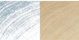
**Medullary Rays** are character marks that appear as “ribbons” running vertically through the tree, perpendicular to the growth rings, allowing movement of sap. When veneer is quarter cut through the medullary rays it produces a flake pattern on veneer that is most notable in White Oak.
