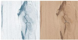
**Knots** form in the wood as a result of cut or broken off limbs or sprout branches. Open knots occur when a portion of the wood substance of a knot has dropped out of the leaf. Tight knots are solid across their face and fixed by growth to retain their place. Pin knots are smaller than an inch, are not easily detectable and do not contain dark centers.
