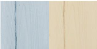
**Mineral Streaks** are natural marks appearing in the form of a dark patches or discoloration caused by the presence of minerals in the soil from which the tree grew.
