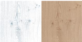
**Pippy** character marks identify veneer that looks like it has a case of the measles—with multiple tiny spots that dot the grain.
