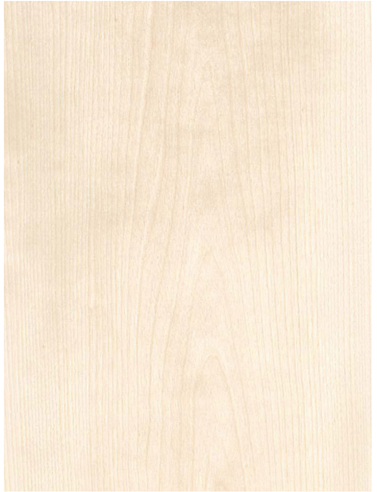
ABOVE: FLAT CUT WHITE BIRCH. BELOW LEFT: WHITE BIRCH IN A SLIP MATCH. BELOW RIGHT: WHITE BIRCH IN A BOOK MATCH.
