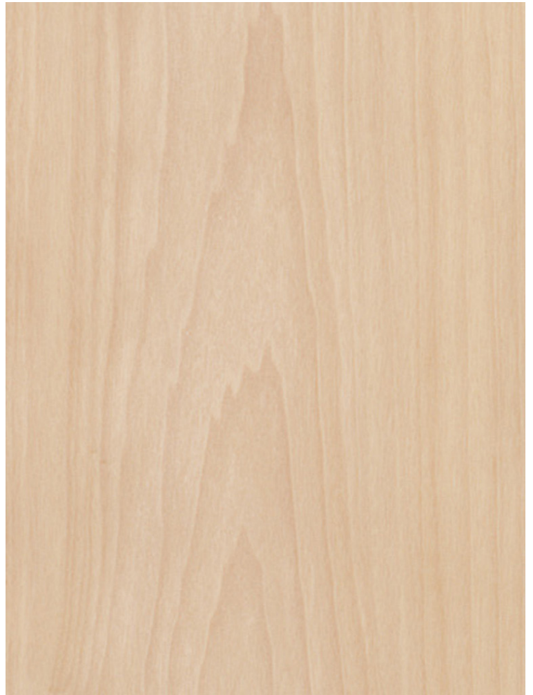
ABOVE: FLAT CUT PLAIN ANEGRE. BELOW LEFT: ANEGRE IN A SLIP MATCH. BELOW RIGHT: ANEGRE IN A BOOK MATCH
